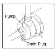
drain plug from the pump. Tip the spa jet unit slightly, until all the water has drained from the pump. Replace the drain plug.
